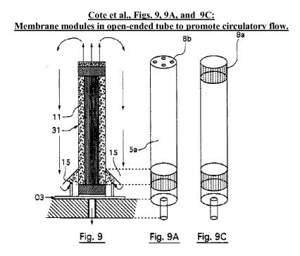
Cote et al. further discloses that this arrangement is used to promote circulatory flow within the tank. Specifically, Cote et al. teaches, "The ozone could thus be produced out of air (applicant's recited aeration generated by an aeration header) or oxygen. . . . [T]he ozone is thus used to serve both as a circulation fluid and an oxidizing fluid." Cote et al., col. 3, lines 10 and 27-28.
